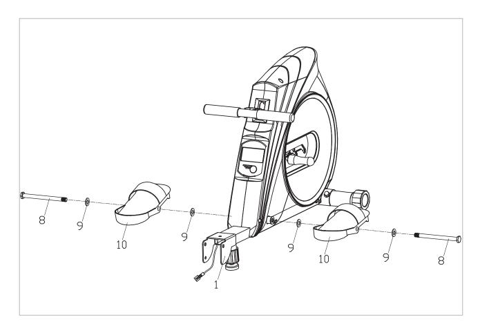
• Attach the pedals (10) to the main frame (1) with the bolts (8) and the flat washers (9).
