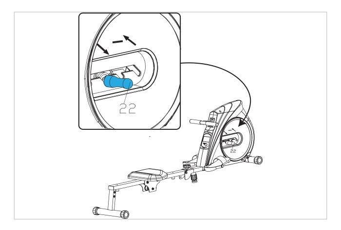
• Pull the handlebar (22) out of the groove as indicated by the arrow, pull the handlebar (22) forwards or backwards, then insert the handlebar into a different groove.
