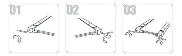
(1) Running belt deviates to left - Start the machine, set speed at 2-3 km/h without a load on the belt, use Allen key to turn the screw 1/4 turn (see fig. 1). Then allow the machine to run without a load for 1-2 minutes. Repeat process until the belt becomes central.
