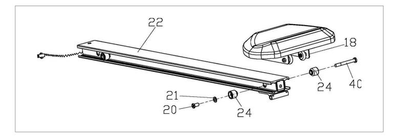
Take off the Cross pan bolt (20), Flat washer (21), Limit valves (24), Limit valves axis (40), then insert the slide rest (18) onto the slide way (22), and then tighten slide rest (18) by Cross pan bolt (20), Flat washer (21), Limit valves (24), Limit valves axis (40).
