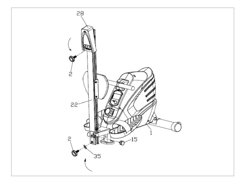
The Rowing machine could be folded if you do not use it. First take off the knob (15), and the knob (2), flat washer (35), then fold the slide way (22) and protective guard (28) as the diagram show. Fix the mainframe (1) to the protective guard (28) with knob (2) and flat washer (35).
