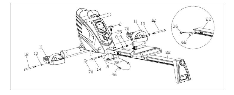
Connect the Sensor wire (46) and the Sensor splice (36), the cable might be hidden inside the slide. Then insert the Stay pipe (66) through a hole in the Slide way (22), Then tighten the slide way (22) to the mainframe (1) with hexagon bolt (14) Flat washer (8) Nylon nut (9) and put the cap (70). At last lock it by Knob (2) and Flat washer (35).
