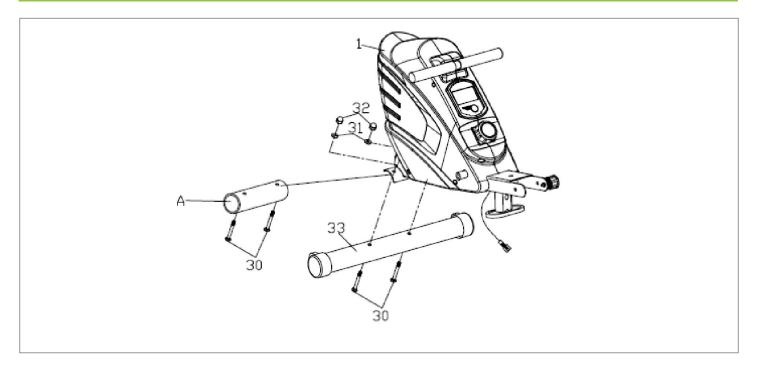
1. Remove the paper tube A ,carriage bolt (30), arc washer (31), and cap nut (32) from the . front bottom tube (33) ;
