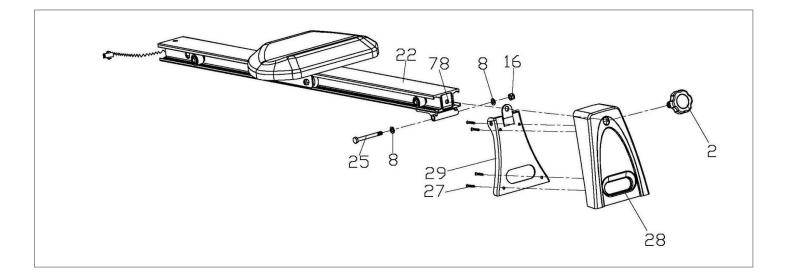
Tighten the stand rail (29) to the Slide way (22) with Hexagon bolt (25), Flat washer (8), Nylon nut (16). Then tighten the protective guard (28) to the Stand rail (29) with Cross pan bolt (27), lock the Stand rail (29) to the L-shape connection strap (78) with Knob (2).
